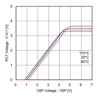
Figure 29. VSP - PCT offset voltage
