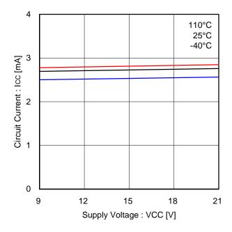
Figure 9. Circuit current
