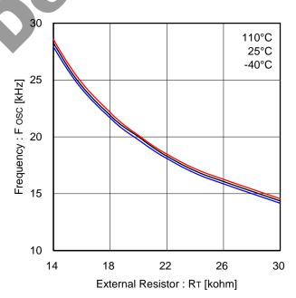
Figure 32. Carrier frequency - RT
