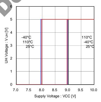
Figure 28. Under voltage lock out (VCC)
