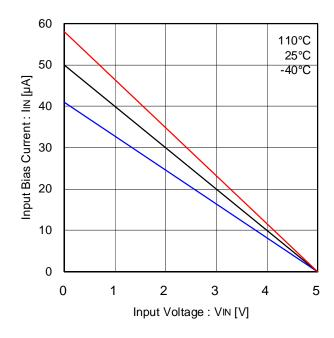
Figure 21. Input bias current (CCW, FIB)
