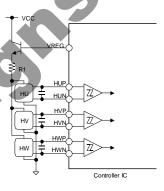
Figure 6. VREG output pin application example
